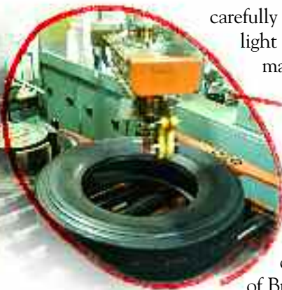
All Bridgestone truck radials have a yellow static balance mark to aid in initial tire balance and mounting.
