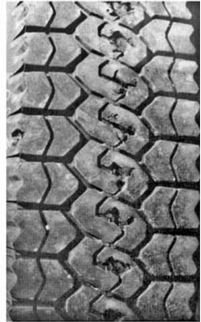
Example of Dyno Damage
